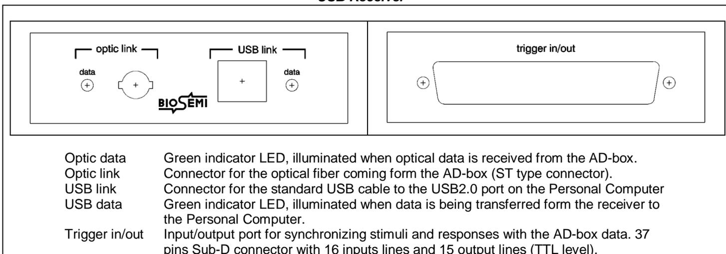
The receiver converts the optical data stream from the AD-box into an USB2 compatible signal to the PC. In addition, trigger input signals are added to the data stream see [http://www.biosemi.com/faq/trigger\\_signals.htm](http://www.biosemi.com/faq/trigger_signals.htm). In addition, the receiver can send output pulses via the trigger port. Finally, the sample-rate frequency is available at the trigger port for synchronization purposes.
